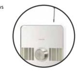
Turn the flow control knob to ensure it moves smoothly (the full range of movement runs from 9 o'clock to 3 o'clock). If not, the knob maybe fitted incorrectly. The shower should be commissioned with the knob in the mid position (12 o'clock).
